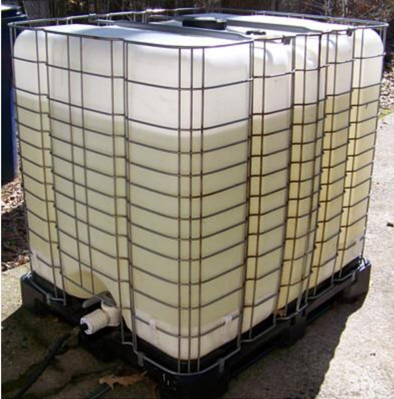
The original tank after cleaning. With over 200 gallons collected, it's obvious the support cage is needed. With 8 feet of 3/4 inch hose connected, the flow rate from the tank (at greater than half full) is over 4 gallons/minute (measured by the time needed to drain 50 gallons from the tank). If you're curious about the flow rate from the 2 inch valve, just be sure to stand to the side when you open the valve...
